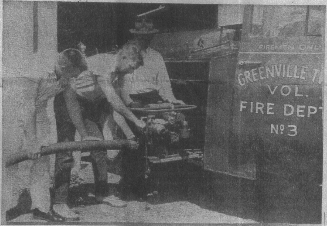
TWO MAN PUMP —Members of the Greenville Volunteer Fire Department demonstrate the operation of the portable two man pump. The body of the tank truck shown above was built at the fire house by a former member of the department. Shown left to right are Bill Burkhardt, Jerry Miller, and Chief Harry Willian.
